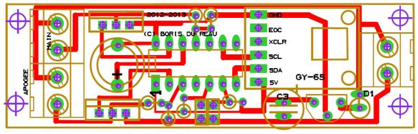
An epoxy board is provided with the kit, all components are drawn so that they can be quickly identified. This is a single sided board. This means that you only need to solder the components on one side.
