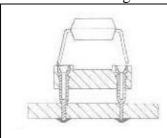
On a new circuit, legs are wider than the socket
