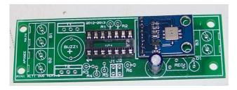
The  $47\mu F$  capacitor has a « + » which should go up, the other leg being connected to the ground at the bottom.
