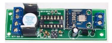
If it has not been done already; cut the connectors so that they are 2 pins. Then plug them to the board. Use cella tape to hold them while you are soldering.
