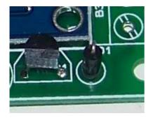
The protection diode has to be correctly plugged. The silver ring should be at the bottom, touching the board.
